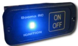
**PRESS** the **Yellow "ON/OFF"** button. IGGY's blue LED will start to flash **faster** indicating that IGGY is ready to arm the ignition circuit. Now, if you have adjusted your receiver channel correctly, switching on the selected transmitter switch/channel will arm IGGY (Ignition state is on) and the LED will be permanently lit. If the blue LED does not light up permanently then you will need to adjust your transmitter. Please refer to your transmitter instruction manual.
