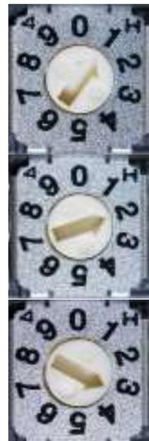
***IMPORTANT: After setting the subtrim of a slave servo to store the setting you must move the rotary dial back to the 0 zero position.***
